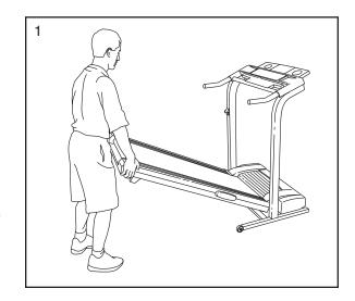
Move your right hand to the position shown and hold the tread knob to the left and hold it. Raise the treadmill until the catch is the latch knob. Make sure that the catch is securely held by
